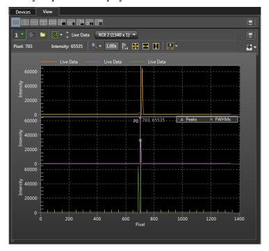
Figure 20. Spectrometer Alignment: Before Rotational Alignment
